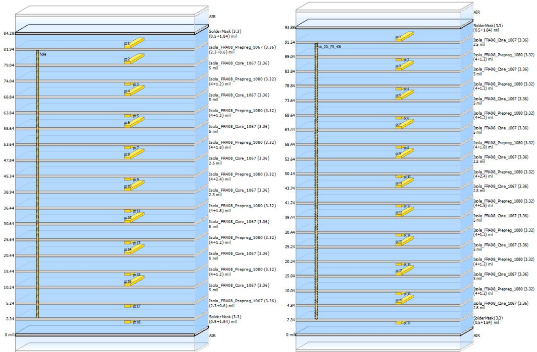
Figure A.10 - Definition of 18L PCB stack-up (left) and 20L PCB Stack-up (right)
