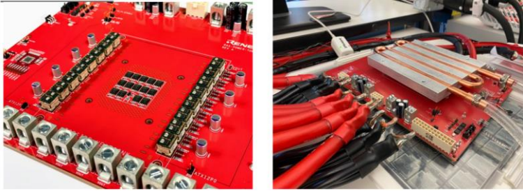
Renesas 16 power tower solution for 1000A
