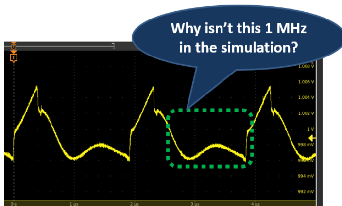
Figure 29 – Measured voltage ripple on the TPS7H4003 EVAL PCB with load.
