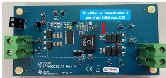
Figure 15 – Depiction of TPS7H4003EVM Evaluation Board
